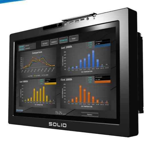
Condition Monitoring by Fincantieri Marine Services North America offers an integrated approach to data collection, communication, projections and analysis. The SOLID combines a monitor, data logger, powerful analysis software and radio (LTE & SAT), all in one compact unit. It is the latest technology designed to meet the most demanding requirements for monitoring and direct data analysis of complex thermodynamic systems.
